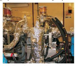
Fig. A.1.2: The sixth RF cavity along with vacuum system during baking.
