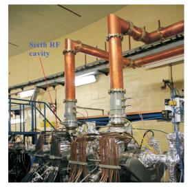
Fig. A.1.1: A view of sixth RF cavity installed in Indus-2.
