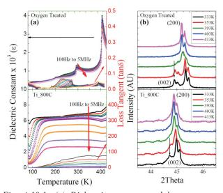
Fig. A.10.1: (a) Dielectric constant and loss tangent vs temperature at various frequencies from 100 Hz-5 MHz for oxygen treated and Ti\_800C samples. (b) Merging of (002) and (200) peak in temperature dependant XRD, is a signature of tetragonal to cubic transition, for the two samples.
