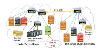
Fig. A.4.1: Architecture of DRS for Indus control system.
