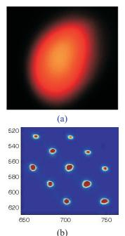
Fig. A.6.4: Recorded  $H^-$  beam spot (not to scale) using (a) fluorescent screen ~ 6 X 8 mm and (b) pepper pot emittance monitor.
