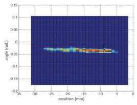
Fig. A.6.3: Recorded  $H^-$  beam emittance using a slit and Harp method, at the centre of LEBT (RMS emittance ~ 25 mm-mrad (un-normalized)) after removal of noise.
