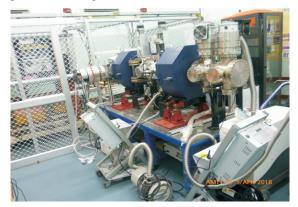
Fig. A.6.1: Experimental setup of  $H^-$  ion source coupled with LEBT and beam diagnostics.
