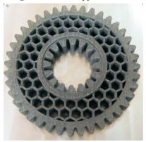
*Fig. L.3.3: External and internal geared geometry with honeycomb core.*
