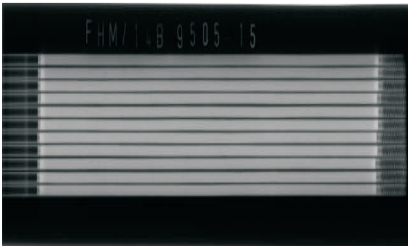
Fig. L.4.1: Digitized image of XGAR film of ten fuel pins.
