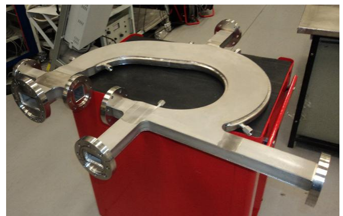
Fig. I.1.3: Photographic image of vacuum chamber for 9.5 MeV linac.
