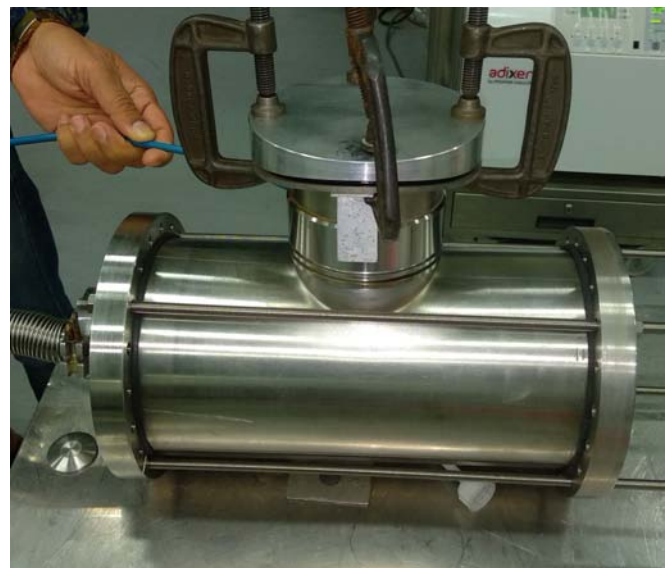
Fig. A.9.3: Leak testing of transition piece.
