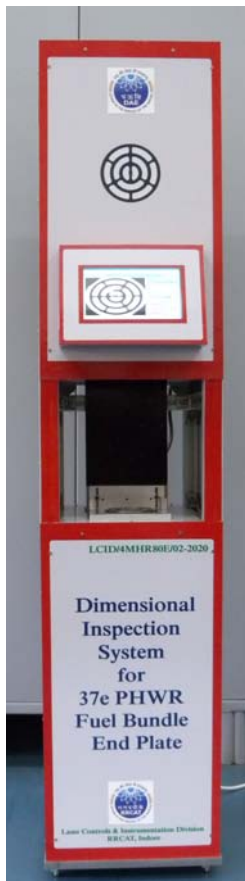
Fig. L.1.1: Photograph of machine vision based dimensional inspection system for PHWR fuel bundle end plate.
