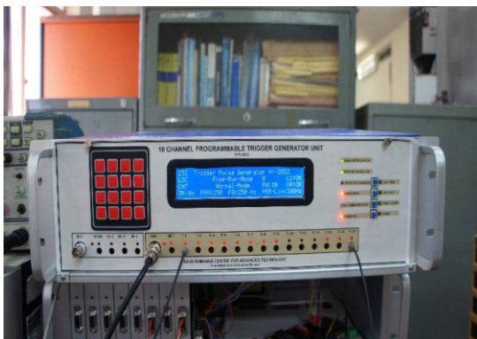
Fig. A.10.1: Snapshot of programmable trigger generator for Linac of EBRPF.
