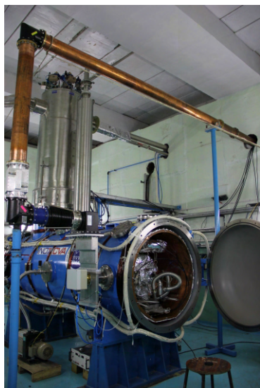
Fig. A.3.1: HTS cryostat with cavity in the vault.
