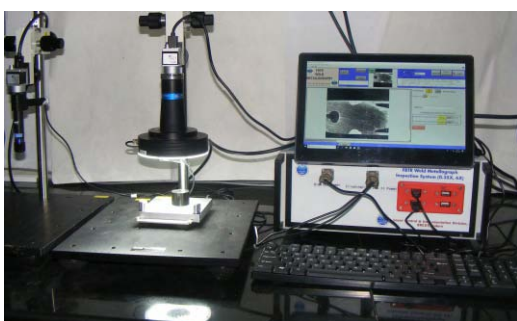
Fig. T.2.18: Machine vision based FBTR weld metallography system with two imaging stations.
