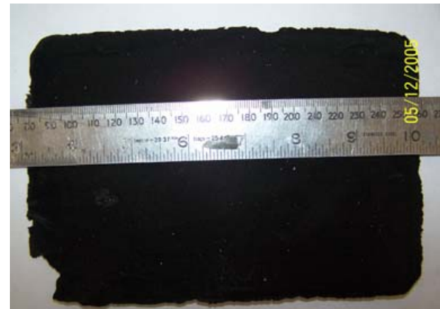
Carbon Foam Electrode ( 125 x 80 mm)
