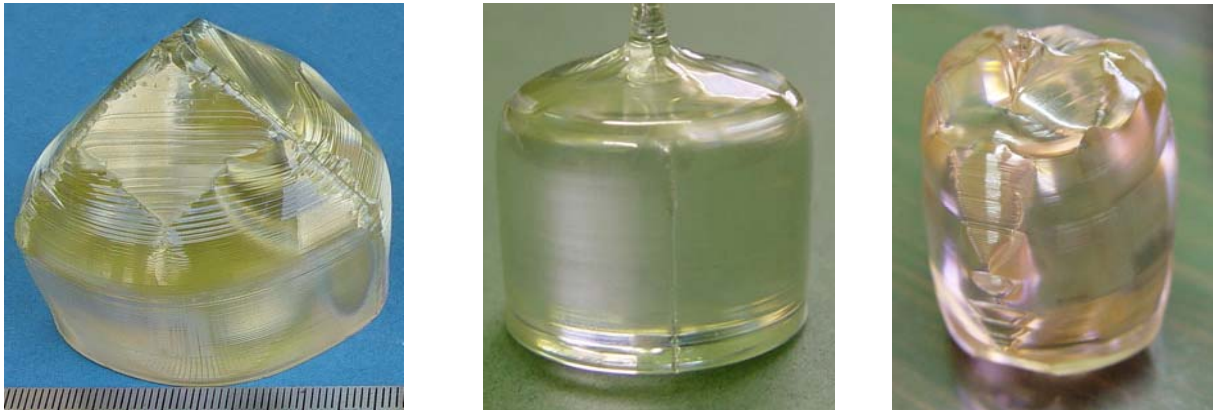
Congruent LN crystals; (a) without doping, (b) with Er (0.25, 0.5 and 1 mol%) and (c) with Zn (2 and 4 mol%) doping grown with the automated system.
