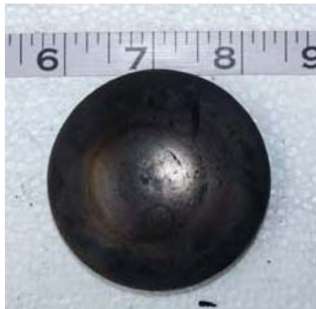
Pt-Loaded Carbon –silica composite cylinders and disc
