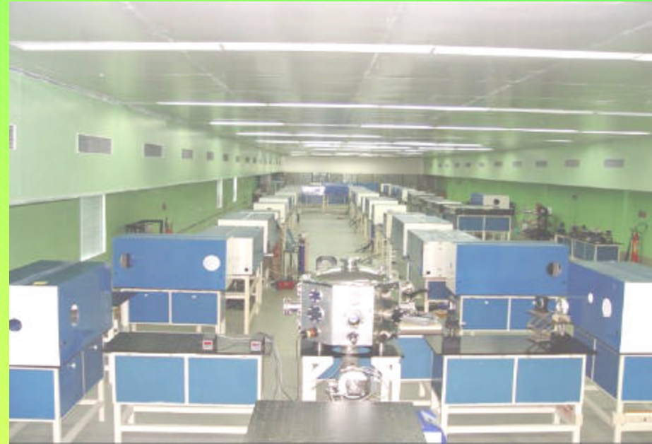
High power Nd:glass laser system
