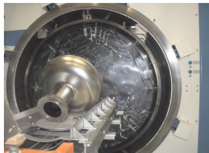
Fig. A.5.2: Cavity loading in furnace
