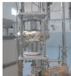
Fig. A.5.3: Cavity mounted on VTS insert
