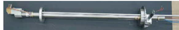
Fig. L.1.1: Laser cutting tool for liner tube and end fitting of 540 MWe TAPS-4 reactor.
