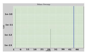
Fig. A.7.3: RGA spectrum of NEG activated chamber.
