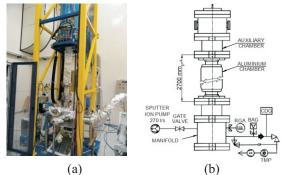
*Fig. A.7.1: (a) Coating setup with vacuum chamber, and, (b) schematic of ultimate vacuum test setup.*
