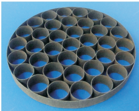
Fig. L.9.1: Mesh type spacers for fuel cluster simulator of 540 MWe PHWR fuel bundle.
