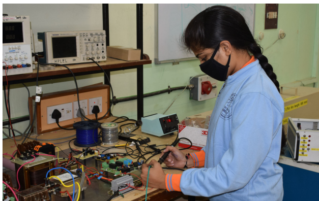
Apprentice carrying out electronic assembly and wiring.
