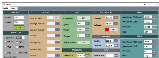
Fig. T.3.4: Screenshot of data logging of various parameters in NEG coating system.
