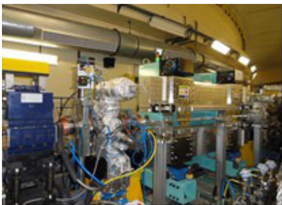
Fig. T.3.16: U1 undulator with NEG coated chamber.
